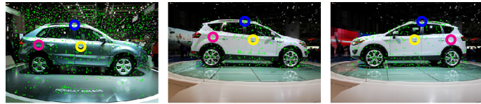
Figure 1: Query features (left) are matched to the class model represented by the two rightmost images. If matching is based on descriptor distance and absolute spatial distance between features, ambiguity still remains. If oriented distances are considered, the correct configuration is favored.
