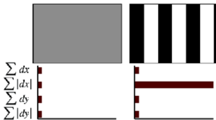
Figure 4 [1]: The sum of absolute values of wavelet response can preserve information of intensity changes in the sub-patches.
