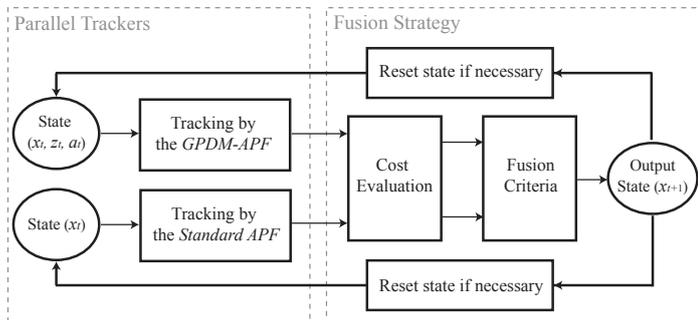
Figure 1: An overview of the fusion framework.
