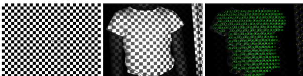
Figure 1: The grid pattern (left). The corners of the squares are ‘grid intersection points’ and there are  $w_{\text{grid}} \times h_{\text{grid}}$  ( $23 \times 28$ ) of these. The grid pattern as projected onto a subject (center), and after identifying grid intersection points (right).
