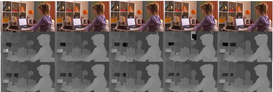
Figure 4. Top Row: 5 consecutive Frames (only left view); Middle Row: the disparity maps estimated frame-independently using the hybrid stereo approach; Bottom Row: the corresponding disparity maps estimated with temporal constraints.
