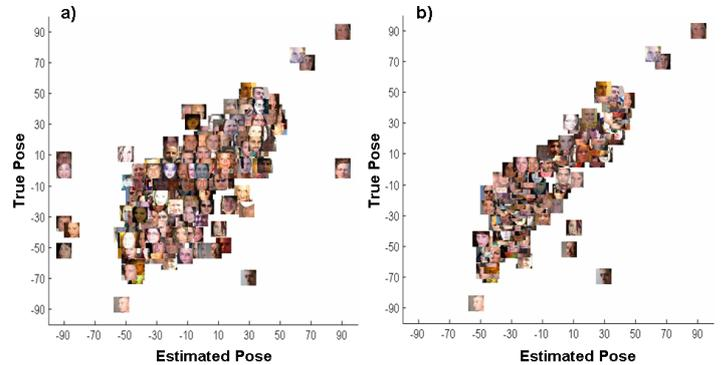
Figure 3: The scatter plot of the results (a) for all of the test data. We achieve a PCC of 0.76 and a MAE of 13.21 degrees and (b) for a subset of the test data uniformly sampled at each true pose. We achieve a PCC of 0.88 and a MAE of 11.72 degrees. The x-axis represents the estimated pose and the y-axis represents the true pose.
