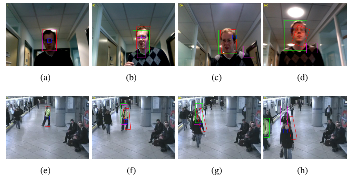
Figure 2: Adaptive multi-feature tracking results with comparisons to other methods. AMFT (green), standard PF (magenta), IVT [4] (red) MS [5] (blue).
