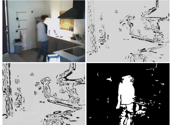
Figure 1: Stable texture regions based segmentation: frame from a sequence (top-left), region stability map (top-right), extracted texture descriptors (bottom-left), segmented foreground (bottom-right).
