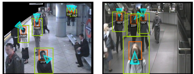
Figure 2: Examples of automated head poses classification of unknown multiple heads in two crowded underground stations. Head candidates are located automatically and head poses are estimated using the proposed method (red dial with pose value).
