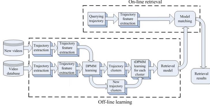
Figure 1: The architecture of the video retrieval framework.
