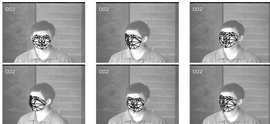
Figure 4: Comparison of the fitted mesh using the SICOV algorithm (dashed line) and the conventional SIC algorithm (solid line) on 6 frames (frame 1, 40, 87, 287, 734 and 767).
