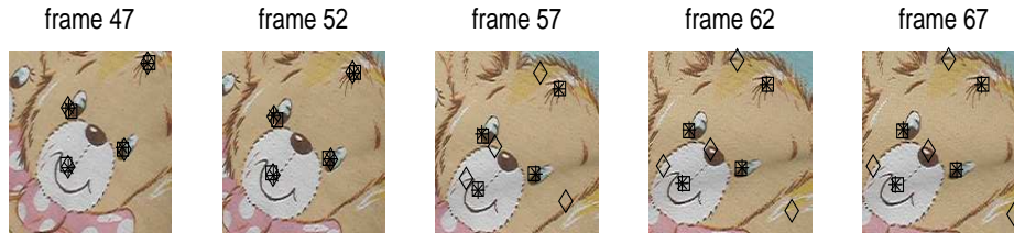
Figure 4: Close-up sequence of 4 point tracks which visible parts (use for training) all ended close to frame number 47. 'True' positions, given by the tracker, are shown by stars. Predicted positions estimated without using the priors are shown by diamonds. Predicted positions estimated with use of the priors are shown by squares.
