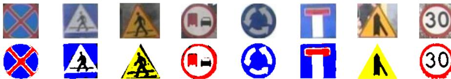
Figure 2: Sample images obtained by sign detector before (above) and after (below) background masking and colour discretisation; 2 bits suffice to encode colours in each image.
