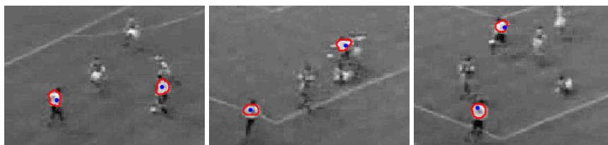
Figure 11: Uniquely tracking multiple similar, noninteracting players. Each object has its own centroid prediction ( blue dot ) and initialization mask but share the same distance penalty. ( Cropped frames shown. )
