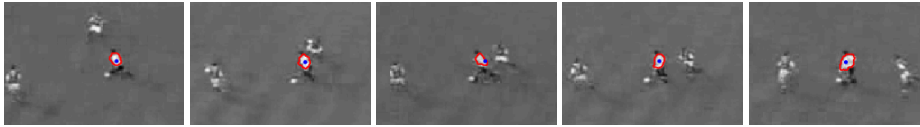
Figure 8: Several cropped frames from the soccer sequence using mean intensity. Blue dot represents predicted centroid.
