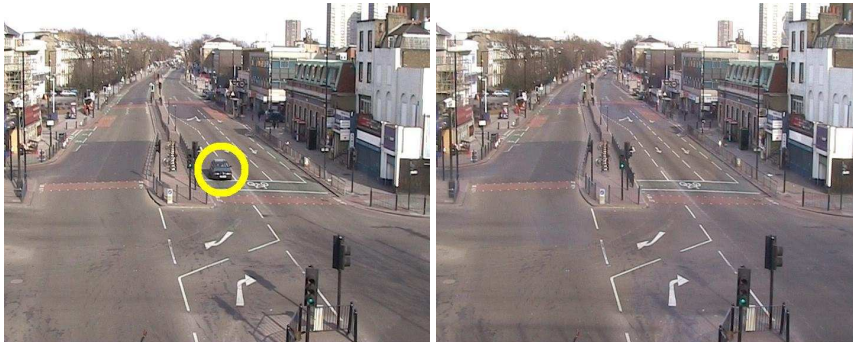
Figure 5: Typical output from the Min-Cut pre-processing stage. Left: Imperfect object removal. Right: Near optimal background recovery.
