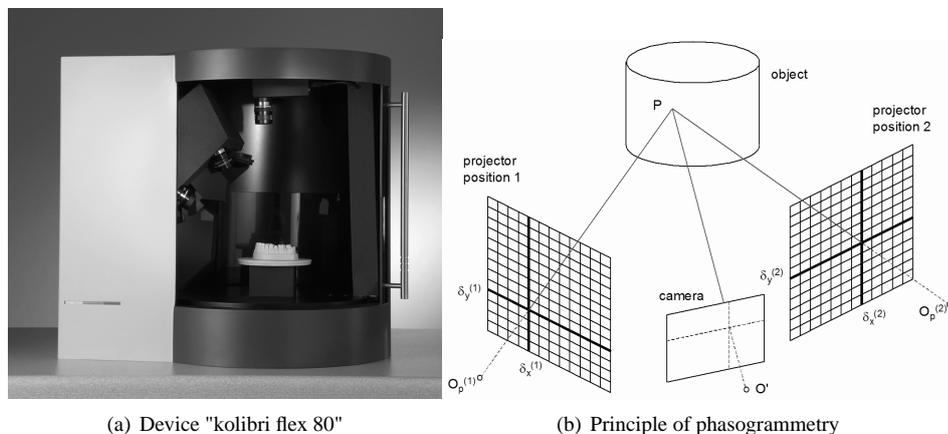
Figure 1: Photograph of the device and measuring principle
