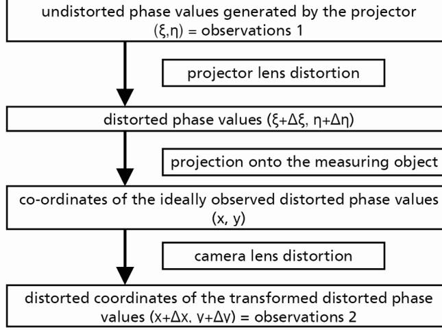
Figure 2: Scheme of the data flow in the systems using fringe projection including lens distortion
