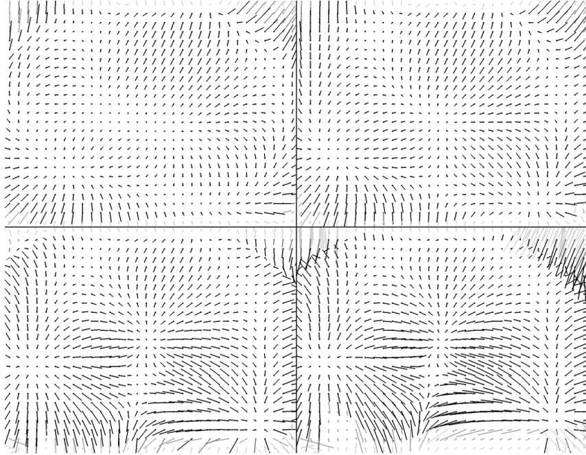
Figure 3: Four of the five different determined layers of distortion of projection unit, device KF1. Upper line: layer1 (left), layer2 (right), lower line: layer4 (left) and layer5 (right). The distortion vectors are scaled by a factor of 100 according to the grid size.
