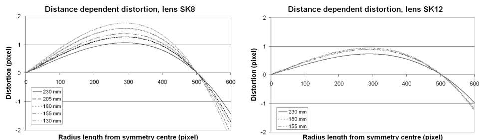
Figure 5: Distance dependent distortion curves of the lenses SK8 and SK12
