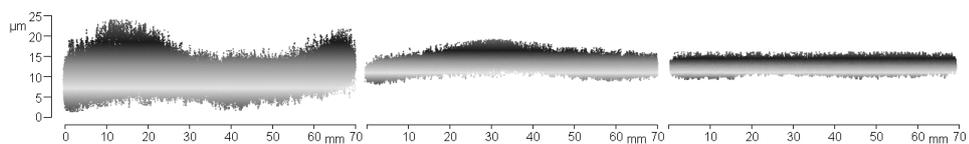
Figure 6: Reconstruction of a plane surface with 70 mm diameter; uncorrected ( $PV=22\mu\text{m}$ ), conventionally corrected ( $PV=10\mu\text{m}$ ), and distance dependent corrected ( $PV=7\mu\text{m}$ ). The Y-axis is inflated by a factor of 1000
