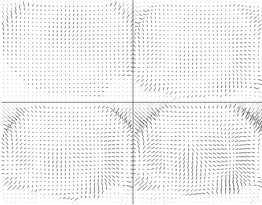
Figure 4: Four of the five different determined layers of distortion of projection unit, device KF2. Upper line: layer1 (left), layer3 (right), lower line: layer4 (left) and layer5 (right). The distortion vectors are scaled by a factor of 100 according to the grid size
