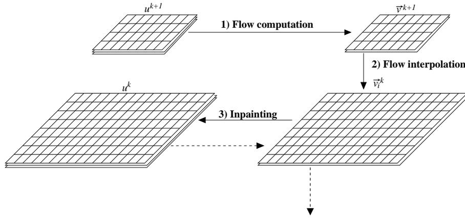
Figure 1: Multiresolution inpainting. From a sequence  $u^{k+1}$  at resolution level  $k + 1$ , 1) the optical flow is computed, 2) it is interpolated at resolution level  $k$  and 3) used to inpaint the sequence at level  $k$ . This process is then iterated at lower pyramid levels.
