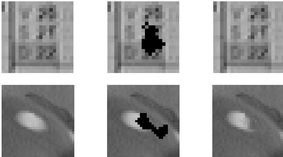
Figure 4: mobcal sequence, details of frame 9: (a) Top left: close-up at a digit inside the calendar. (b) Top center: blotch on that digit. (c) Top right: almost perfect reconstruction. (d) Bottom left: close-up at a white patch on the ball. (e) Bottom center: blotch. (f) Bottom right: partially failed reconstruction.
