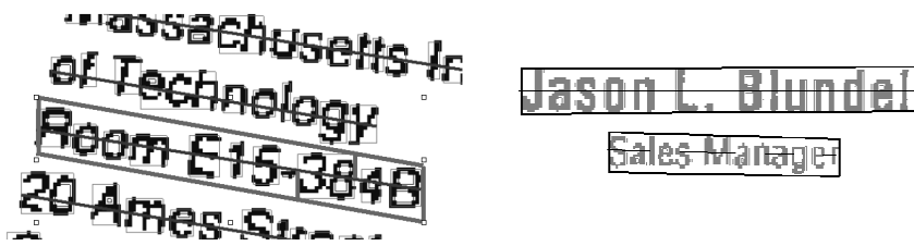
Figure 4. Determination of the bounding box for skewed text (left) and the occasional problems with determining the skew angle merely from the bounding parallelogram (right).
