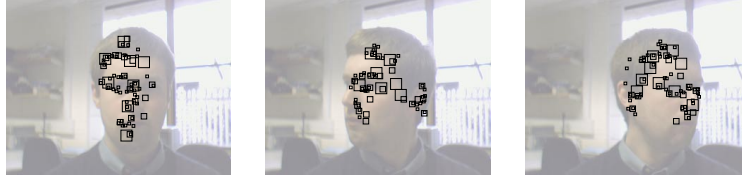
Figure 2: Multi-scale interest points detected in the image region underlying the projected model.
