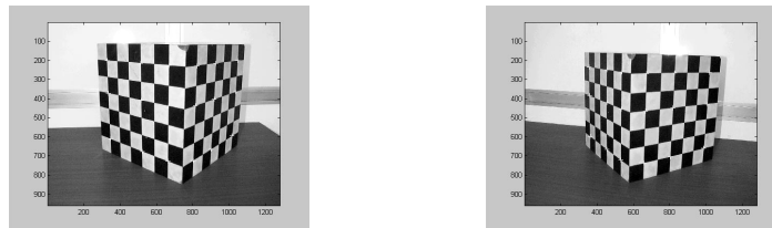
Figure 6: Two images of a calibration object taken by digital camera
