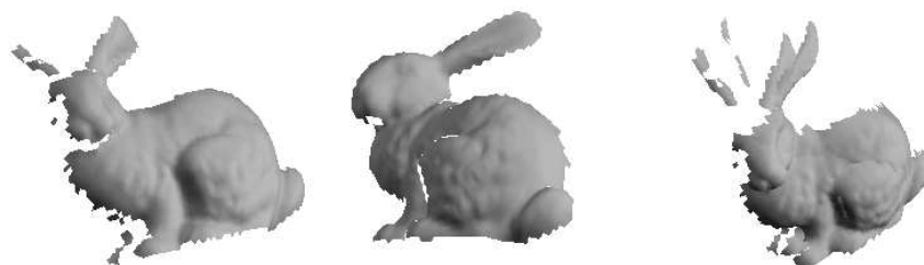
Figure 3: The bunny dataset. (a) shows the scene and (b) shows the model, (c) shows the resulting registration
