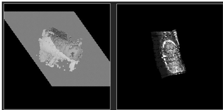
Figure 6: Cross-section of a reconstruction, *with* registration, of an organ phantom. The surface reconstruction (left image) is the same as Figure 5(f). The cross-section is at the same location as in Figure 3. The two ellipses have been aligned.
