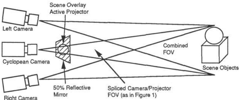
Figure 2: Ideal Stereo Head Configuration for DVF
