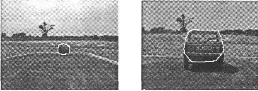
Figure 2 segmented images at ranges of 22.5m and 6.5m
