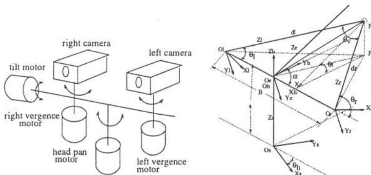
Figure 1: The structure of the robot head and its coordinate frames
