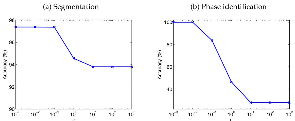
Figure 6: (a) Mean segmentation accuracy and (b) Mean phase identification accuracy with a wide range of  $\epsilon$  in Eq. (12).
