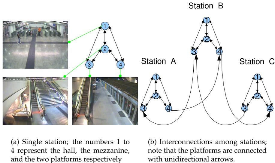
(a) Single station; the numbers 1 to 4 represent the hall, the mezzanine, and the two platforms respectively
